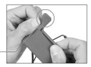
5. Wrap cable management strap around the cable and push tail through loop to secure. Repeat for other earcup. Ensure that the cable is on the outside of the headband attachment arm.
