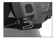
NOTE: If you have both the boom microphone and mask mic connected to the headset, both will be active at the same time. Depending on your environment and operational need, disconnect the boom microphone and stow if you need it to be inactive.
